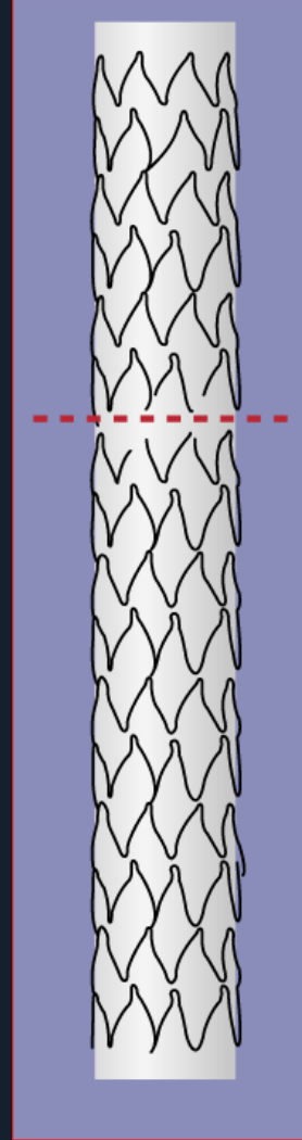
Multiple stent fractures; complete transverse linear fracture
