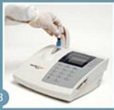
3 When prompted, insert the tube onto the assay device needle.
