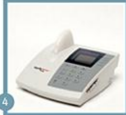
4 After inserting the tube, close the cover and read results within 2 to 5 minutes.
